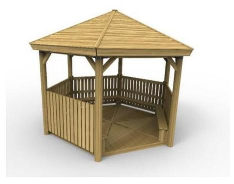
This has an inside diameter of 5.7m, with a total diameter of 6.1m including the overhanging roof. The uprights are 2.63m apart and the Gazebo includes bench seats on five sides (total seating length of approximately 12.5m – capacity approximately 25 children), with 1.1m high palisade balustrades. - The roof is 2.2m high at the outside, rising to 3.7m at the apex.
